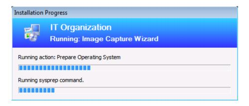
25) After sysprep has completed , the computer will restart automatically and boot using the boot image that was configured for the capture media :
